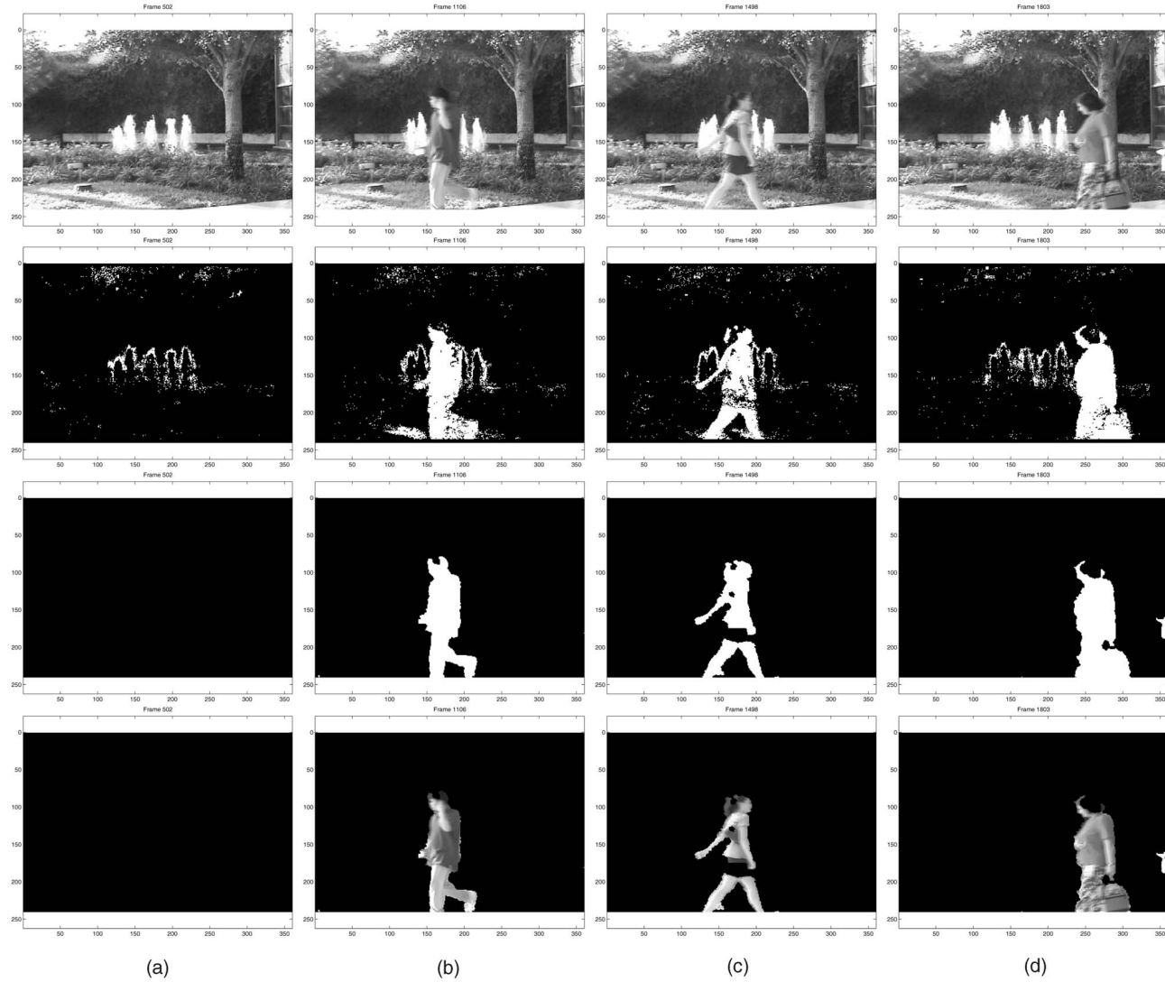
Fig. 10. Fountain Sequence. Background Subtraction in the presence of dynamic textures. There are three sources of nonstationarity: 1) The tree branches oscillate, 2) the fountains, and 3) the shadow of the tree on the grass below. The top row are the original images, the second row are the results obtained by using a five-component, Mixture of Gaussians method, and the third row results obtained by the proposed method. The fourth row is the masked original image. Morphological operators were not used in the results.
