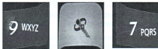
Figure 2. Defective pattern of keypad
