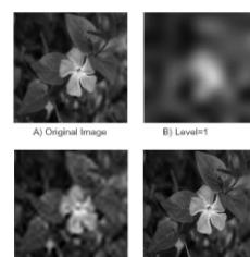
The experiment is also performed for large number of uniform data such as flower image with size of 512  $\times$  512. PSNR(20 log(255/RMS)) is used as an error metric for image compression. High quality reconstructed image of 31.93dB is obtained with 18.24:1 of compression ratio at the level 5 in Fig. 10.
