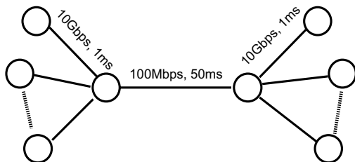
Figure 1. The network topology with simple bottleneck link.
