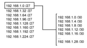
To maximize this address space, the 192.168.1.0 /27 subnet is subnetted further using a 30-bit mask. This creates subnets that can be used on point-to-point links with minimal waste, because each subnet can contain only two possible host addresses.
