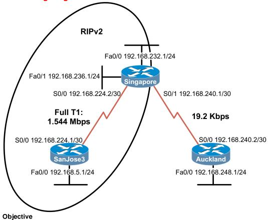
In this lab, you configure a combination of advanced routing features to optimize routing. These features include distribute lists, passive interfaces, default routes, and route redistribution.
