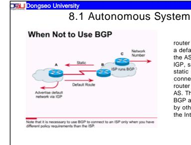
router A is advertising a default network into the AS through a local IGP, such as RIP. A static route affords connectivity through router B to the ISP's AS. The ISP is running BGP and is recognized by other BGP routers in the Internet.
