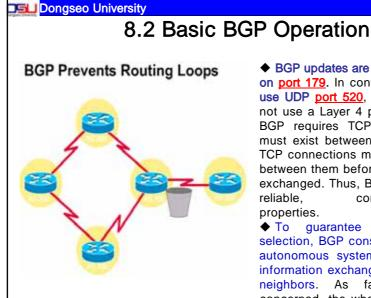
◆ BGP updates are carried using TCP on port 179. In contrast, RIP updates use UDP port 520, while OSPF does not use a Layer 4 protocol. Because BGP requires TCP, IP connectivity must exist between BGP peers, and TCP connections must be negotiated between them before updates can be exchanged. Thus, BGP inherits TCP's reliable,
