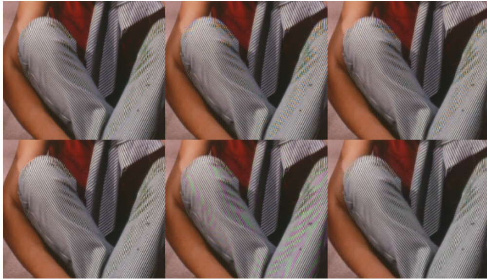
Fig. 1. From left to right and top to bottom: A small portion of the “Barbara” image demosaicked by different algorithms: original image, POCS [4], Successive Approximation [6], Homogeneity Directed interpolation [2], Spatio-Spectral CFA [3] and our proposed method.
