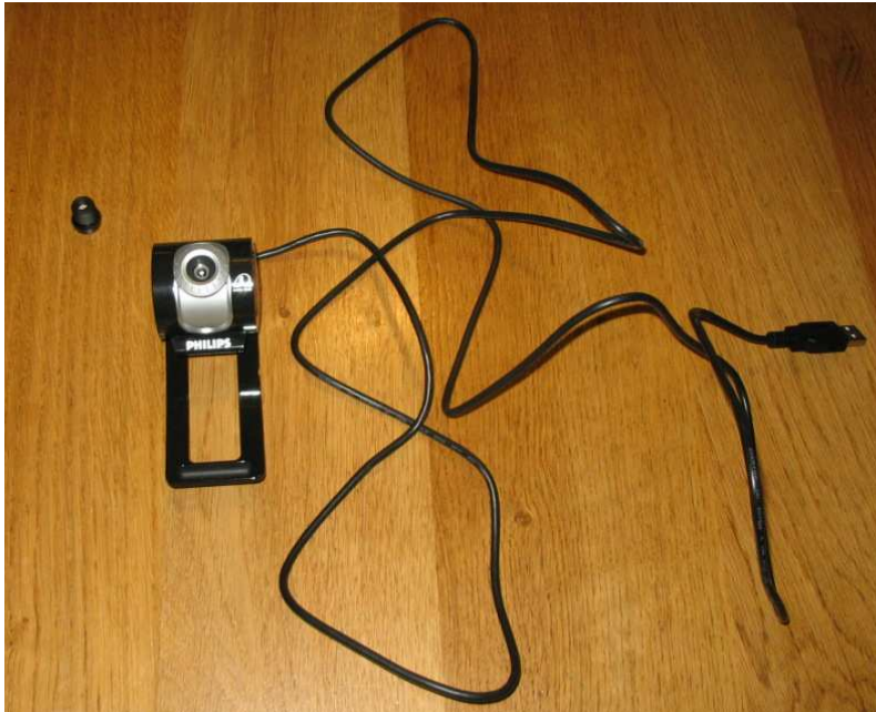
Image 4 : The 4.3MM CCTV Camera board Lens IR DVR without IR-block filter and Philips SPC900NC webcam.
