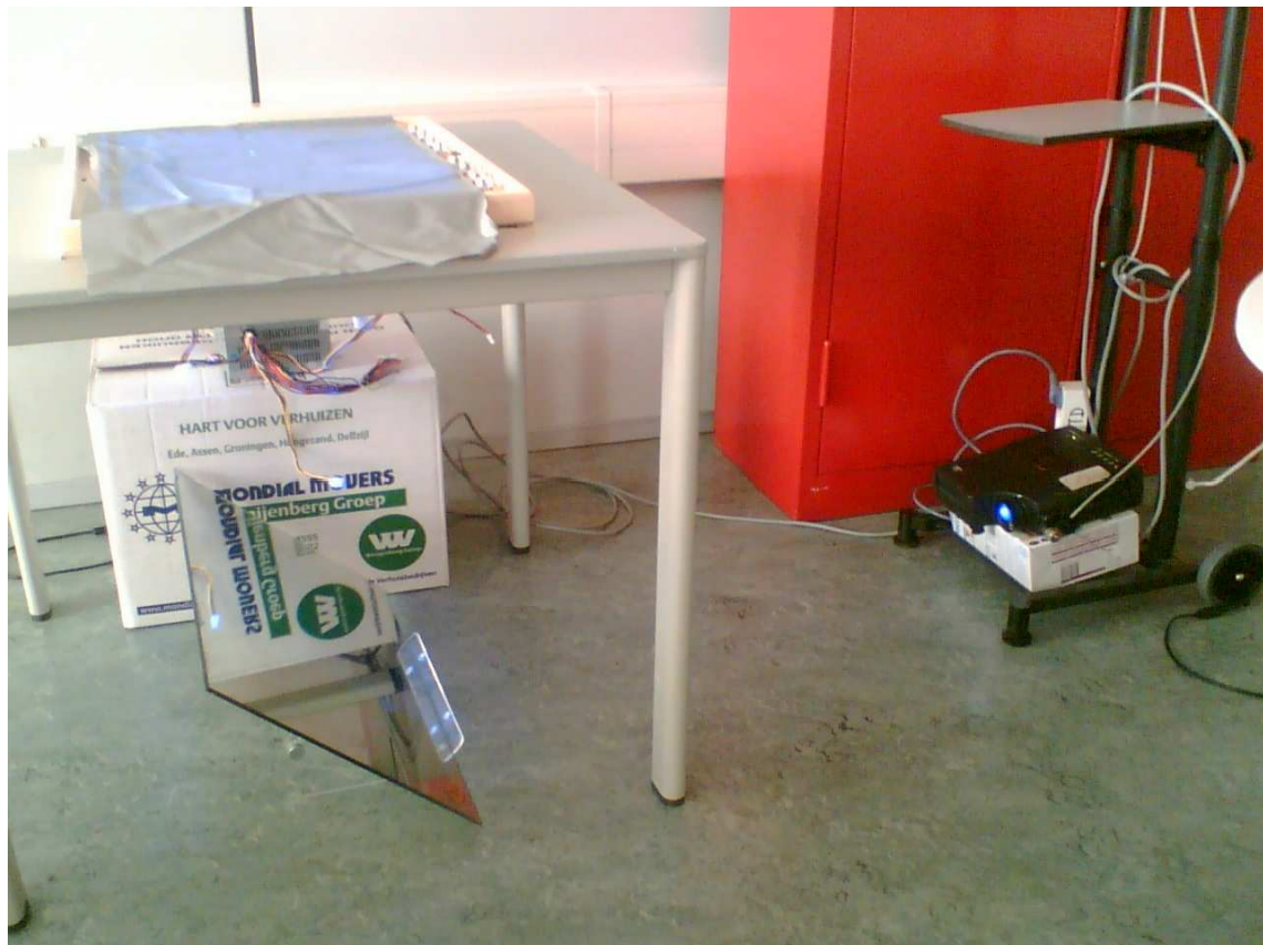
Image 32: Redirecting the beamed image with a mirror.
