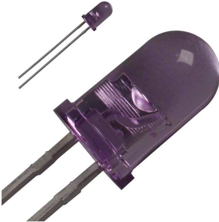
Image 21: An Osram SFH485 IR LED
